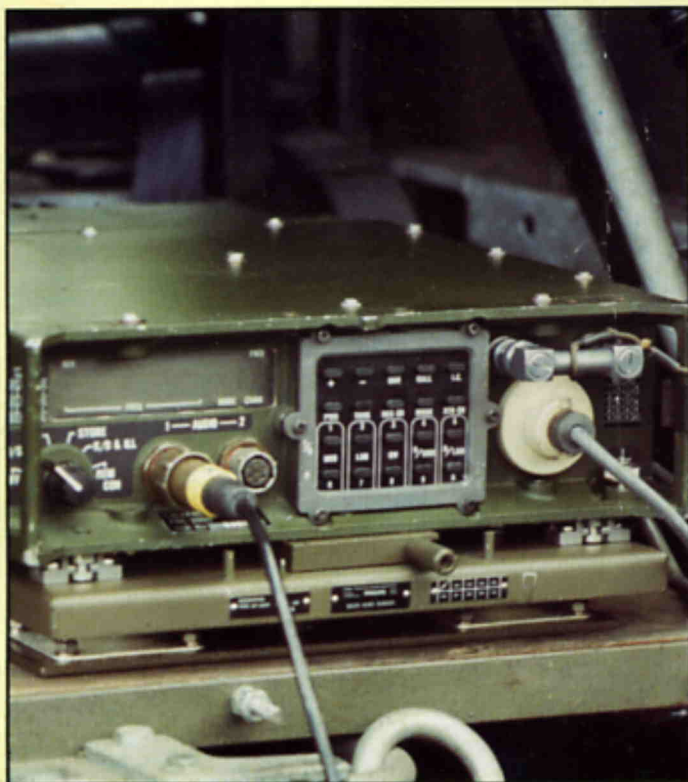
1 CALLPAC covers the HF band from 1.6 MHz to 30 MHz with 284,000 frequencies available at 100 Hz spacing.
